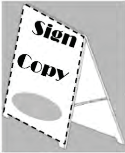
Figure 506-11 Faces that are not parallel, angle \geq 45 degrees
