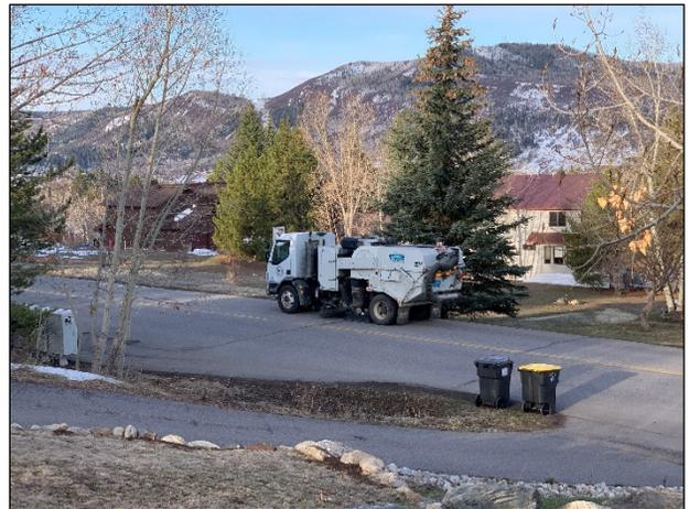
The city utilizes two very different sized machines in its sweeping arsenal. The smaller Sentinel Sweeper is an all-season street sweeper while the larger TYMCO DST-6 Regenerative Air Sweeper is a heavy-duty powerhouse with twice the capacity. Both vehicles collect heavy dirt, sand, gravel, and scoria and are able to follow the contours of uneven road surfaces in dry or wet conditions.
