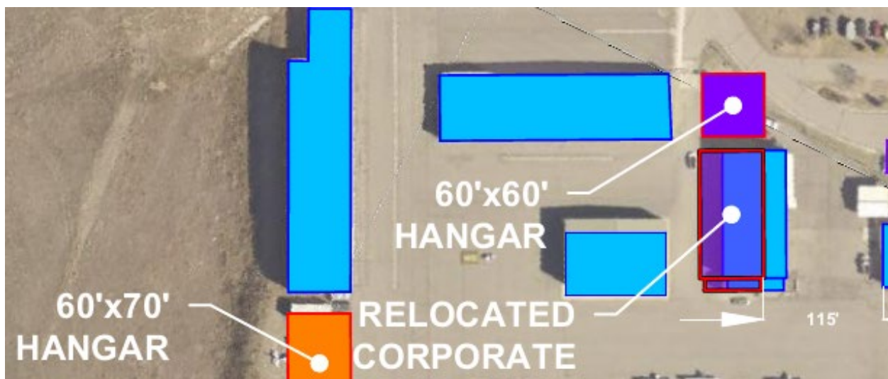
Figure 4.1: Alternative 1.A – Terminal Hangar Development Area: Corporate Hangar Relocation and North Ramp Development
