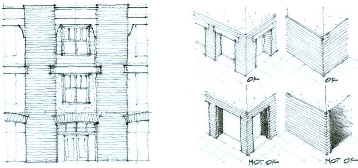
*Figure 2— Buildings shall be visually and structurally anchored with masonry elements at the base level to provide a sense of permanence (left). Base level masonry elements shall be functional parts of the vertical load-bearing structure of the building (or appear to be so), not “tacked on” (right).*
