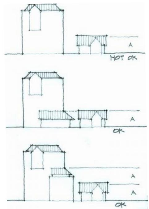
*Figure 5— New developments that are significantly larger than adjacent existing development shall use variations in height and/or mass to provide a more gradual*
