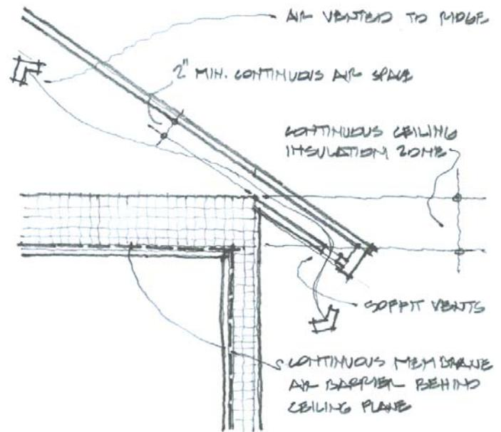
Figure 11— Cold roof deck features.
