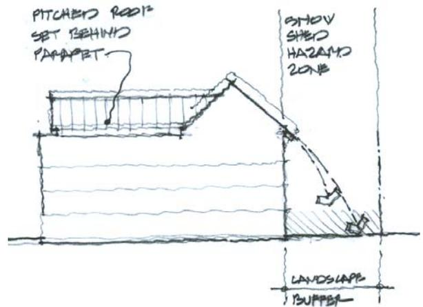
*Figure 9—Pitched roof forms may be set behind a parapet wall where snow may be retained and removed or designed to shed in a defined area away protected from pedestrian and vehicular traffic.*
