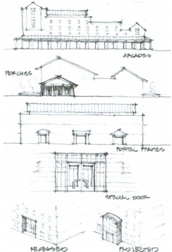
*Figure 3— Primary building entrances shall be clearly distinguished through the use of the above architectural features.*
