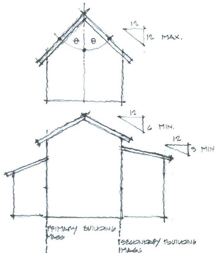
Figure 7— Pitched roof forms shall have a slope of between 6/12 and 12/12. Shed roof forms shall have a slope of between 3/12 and 12/12.
