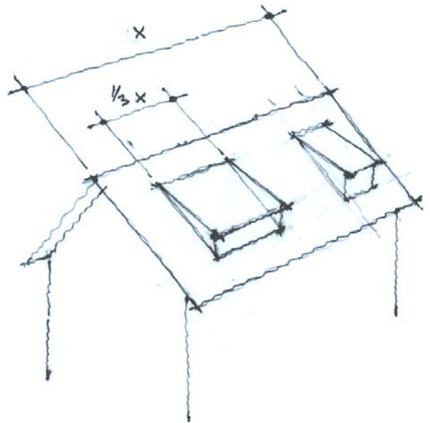
*Figure 8—Any single dormer element shall not be longer than 1/3 the total length of the associated sloping roof plane*
