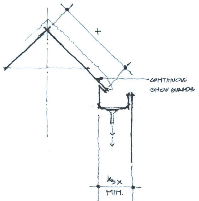
*Figure 10—Flat-roof snow catchment and control areas shall be no less than an area 1/3 as wide as the tributary pitched roof surface.*
