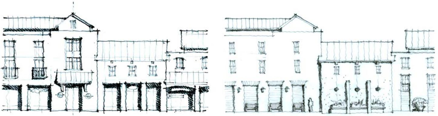
*Figure 4—To the maximum extent feasible, building entrances, retail storefronts, and other active spaces shall be oriented towards adjacent streets, public plazas, and pedestrian walkways (left). Where a direct connection cannot be made between interior and exterior spaces for programmatic reasons, building walls shall be articulated at ground level using a variety of architectural features to provide pedestrian interest (right).*
